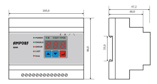
The device is mounted on a DIN rail 35 мм.
