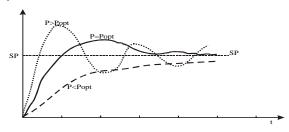
➤ Integral coefficient. If its value is less than optimal, then are obtained small fluctuations in steady state mode. If the
