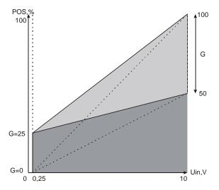
The figure shows the change of the amplifier characteristic by adjusting the trim of the offset (Z), at two values of the trimmer for the gain (G) - 100% and 75%.
