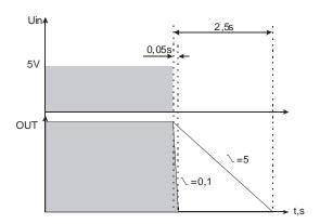
The figure shows the change in output over time when changing the reference from 0V to 5V, at two settings of leading edge trimmer ( $\int$ )- 0,1s and 5s.
