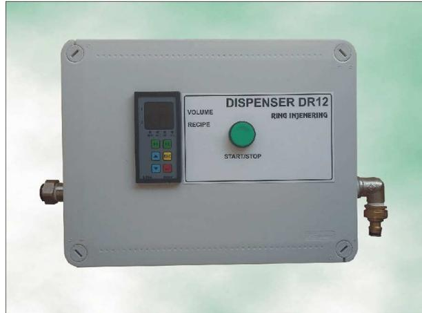
DR12 is the device used to dispense certain amount of water. The start of dosing begins by pressing the green button. The device opens the integrated valve and measures the amount of passing water. Upon reaching the assignment the valve closes and stops the water. DR12 supports 30 pre-stored quantities (programs) for dosing.
