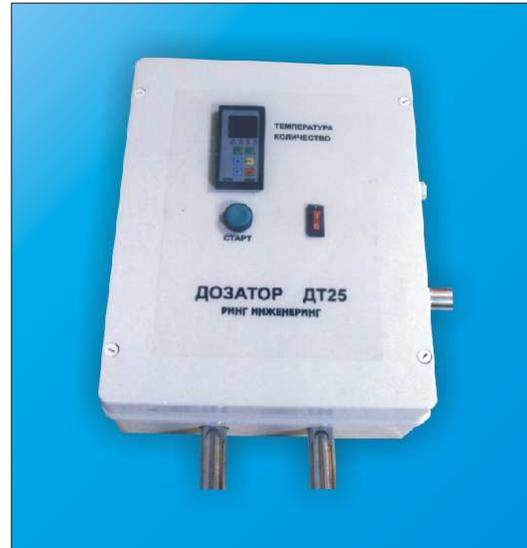
DT25 is the device used to produce certain amount of water to a certain temperature. This is accomplished by mixing of hot and cold water in a separate vessel, installed downstream of the device. DT25 calculates how many liters of hot and cold water must be mixed together in order to perform the job. Water inlet and outlet are connected to the dispenser with established water supply installation.
