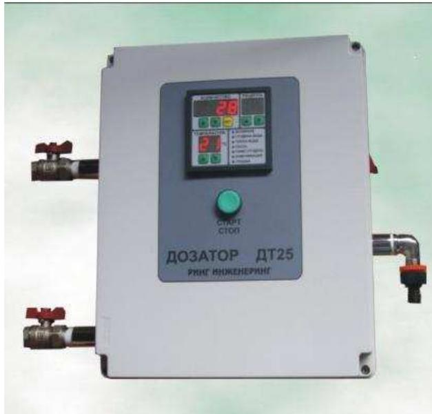
DT25R is the device used to produce certain amount of water to a certain temperature. This is accomplished by mixing of hot and cold water in a separate vessel, installed downstream of the device. DT25R calculates how many liters of hot and cold water must be mixed together in order to perform the job. Water inlet and outlet are connected to the dispenser with established water supply installation.
